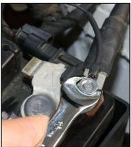
6. Locate the <u>connector with 2 wires attached directly to the negative battery post</u>. Slide the red plastic locking piece on the connector about 1/8" (3 mm) to the left until it stops.
