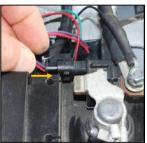
9. Apply the supplied Velcro patch to the rear of the battery outer black plastic box. Press the module onto the Velcro patch.
