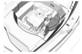
Remove the two battery cover bolts and lift off the battery cover.
