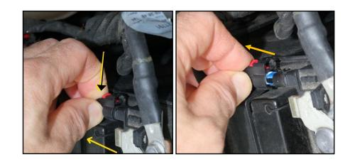
7. Now plug the SmartStopStart GM II module in between each of the two separated connector halves in the vehicle.
