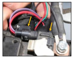
9. Use a supplied tie-wrap to secure the hanging connector body to a nearby cable.
