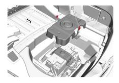
3. Locate the battery negative terminal with the battery sensor. Your battery may appear different than the photo.
