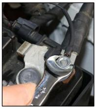
5. Locate the <u>connector with 2 wires attached to the negative battery post</u>. Slide the red plastic locking piece on the connector about 1/8" (3 mm) to the left until it stops.
