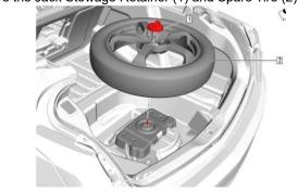
Remove the Jack Stowage Retainer (1) and Spare Tire (2).
