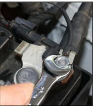
6. Locate the connector with 2 wires attached directly to the negative battery post. Slide the red plastic locking piece on the connector about 1/8" (3 mm) to the left until it stops.
