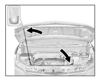
3. Locate the battery. The battery is under the hood on the driver's side. The battery may differ from the photo.
